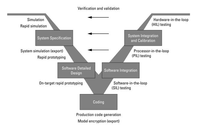
Depending on your application and its role in the process, you might focus on one or more of the steps called out in the V-model or repeat steps at several stages of the V-model. Code generation technology and related products provide tooling that you can apply to the V-model for system development. For more information about how you can apply MathWorks code generation technology and related products provide tooling to the Vmodel process, see:
